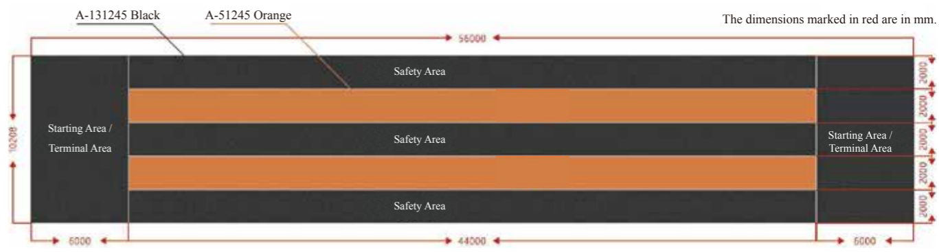
Parkour Track: Total length: 56m, width: 10.208m, track length: 44m, track width: 2m, safety zone length: 44m, width: 2m. Wide: 4.5cm
